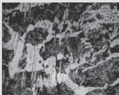
Figure 6.2 Typical microstructures of iron (400×). (From Metals Handbook , 9th ed., Vol. 1, American Society of Metals, Metals Park, Ohio, 1978.)
